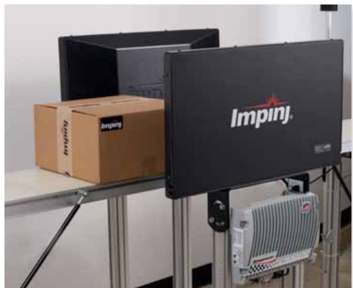
Figure 4: Bulk encoding method for encoding direct apply tags
