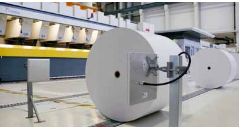
Picture 4. Paper rolls are identified on the conveyor after winding phase
